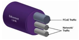
Figure 1 DCB enables multiple traffic type over a single link
